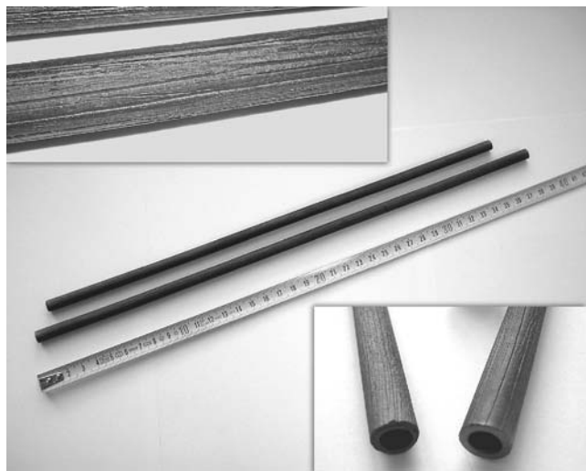
Fig. 16 Dense (\text{SrFe})_{0.7}(\text{SrAl}_2)_{0.3}\text{O}_{3.3-\delta} membranes fabricated from the powder synthesized by method 2. Insets illustrate surface morphology of the membranes
